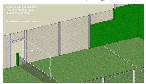
2) With two lateral accesses per side the openings must be a minimum of 0.72 x 2.00 m and a maximum of 1.00 x 2.20 m (See diagram).
