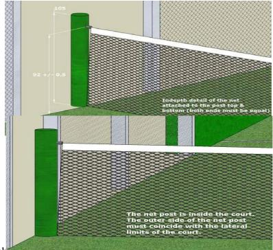
The outer side of the net posts should coincide with the lateral minus of the court, (opening, entrance or metallic fence). They may be circular or square but must have rounded edges.
