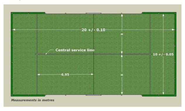
Minimum height must be 6 metres throughout the court. With no elements (i.e. spotlights) which obstruct this area. As for the new facilities it is suggested that the minimum free height should be of 8 metres throughout the court, with no elements of obstruction in this area.
